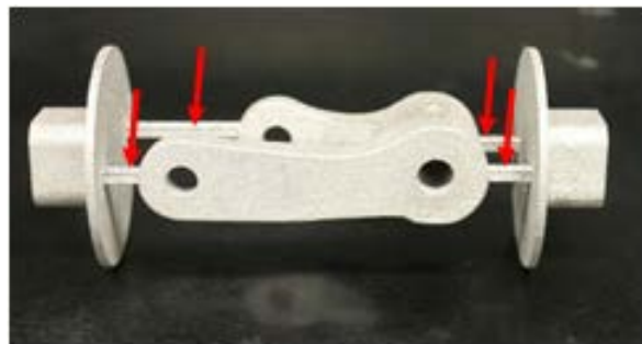
Figure 8. Sacrificial supports along axis of rotation (highlighted by red arrows)
