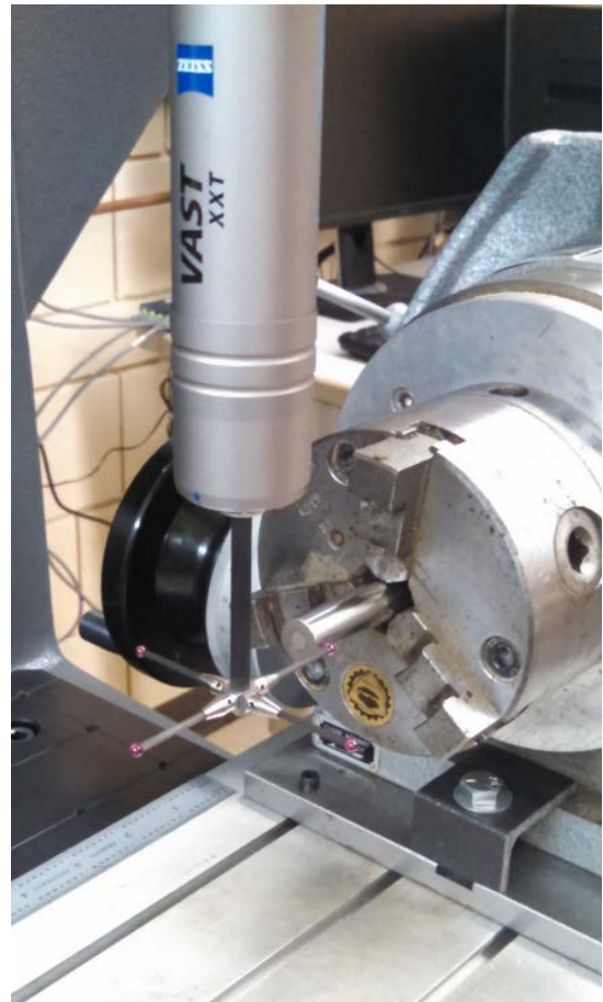
Figure 47. CMM and gage blocks used to measure coaxiality of chuck jaws
